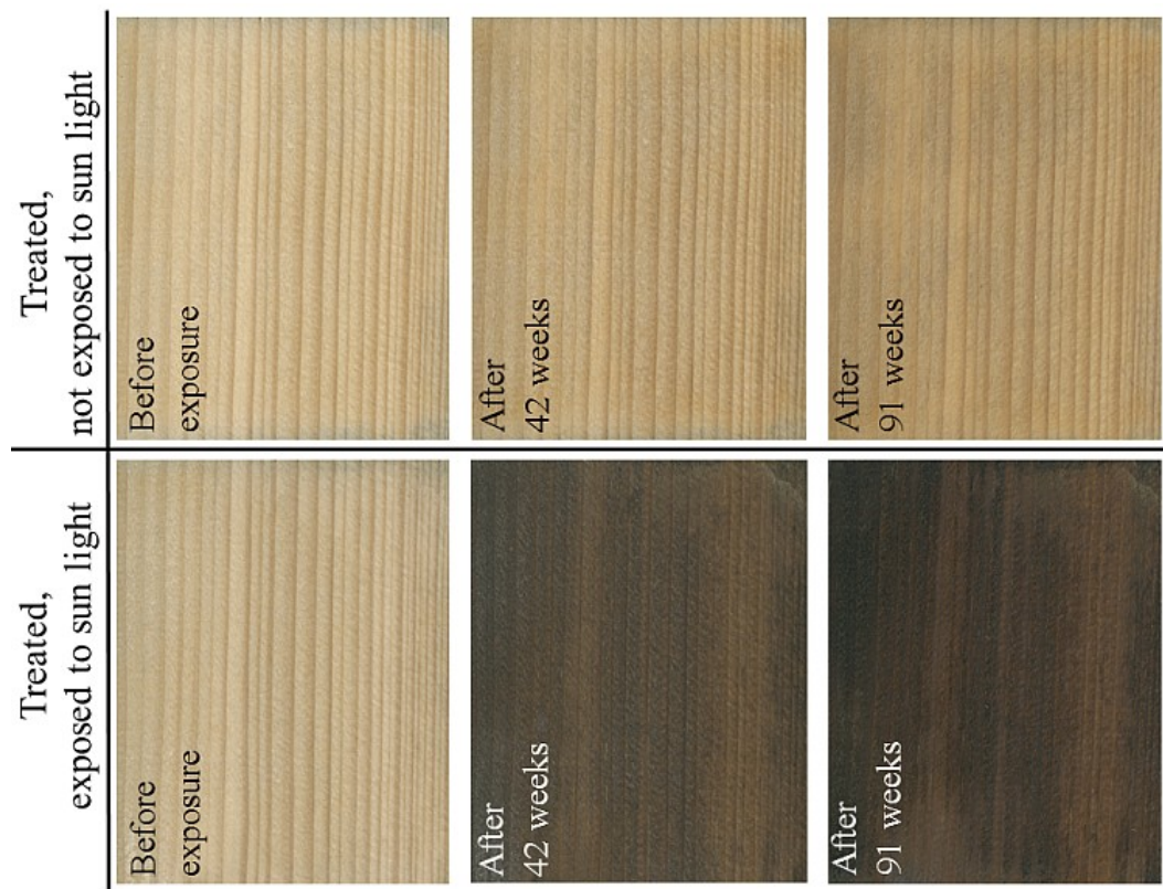
Figure 5. Scans of the specimens of set 2 treated with iron (II) sulfate before and after 42 and 91 weeks of exposure. Upper row = not exposed to sunlight, lower row = exposed to sun light.
